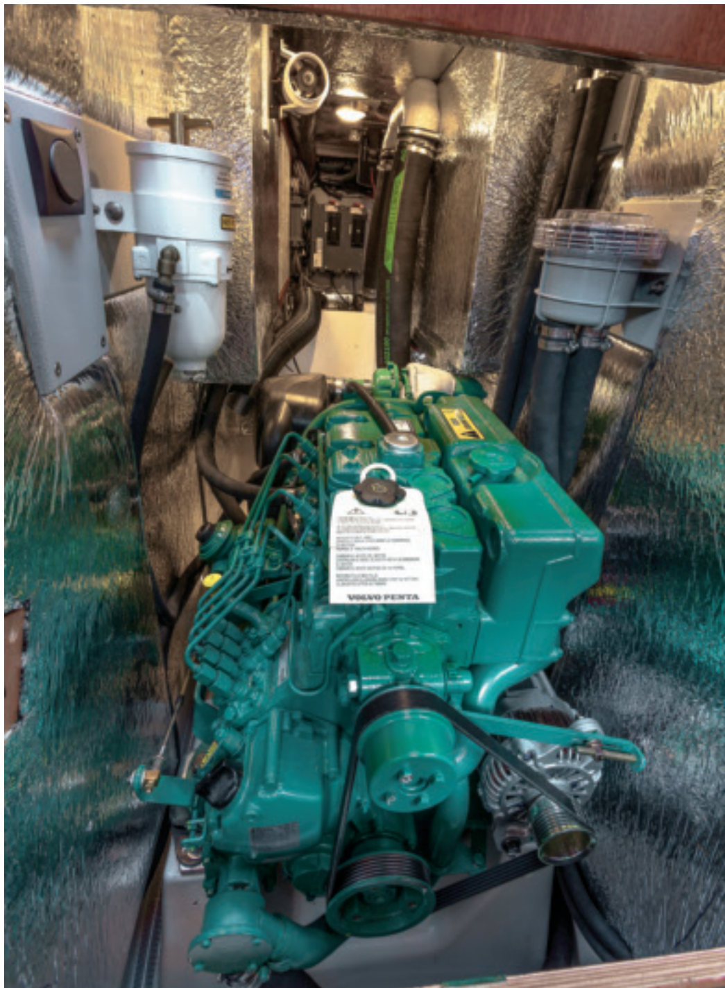
A powerful 75 HP Volvo Penta D2-75 engine
